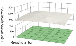
Light distribution profile of 16 FL300 Sunlight in a 4.2 m<sup>2</sup> chamber. Average light intensity 947  $\mu$ mol/m<sup>2</sup>/s ± 4% STDV
